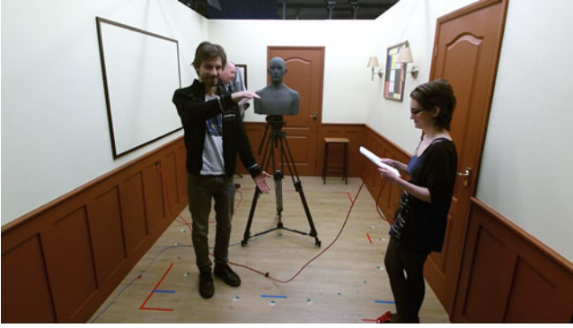
Fig. 8. A sample image in Sequence 3 from Kinect’s viewpoint. Actor (only the head can be partially seen) stands on the back corner while Actress stands in front. An additional subject is clapping his hands for synchronisation of the depth and audio streams.
