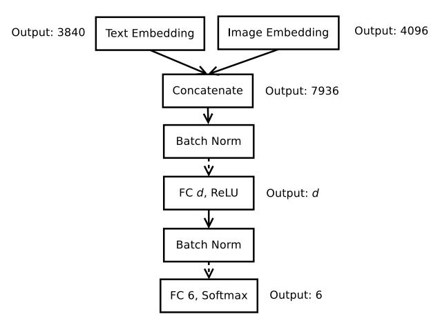
Figure 4.13: Fusion Module (FM): the proposed method for early fusion of textual and visual information. Dashed lines indicate dropout was applied. The hyperparameter d is the number of units in the first fully connected layer.
