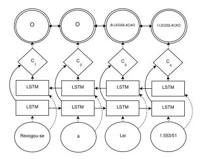
Figure 3.2: The biLSTM-CRF model. The word vector representations serve as input to a bidirectional LSTM layer.  $C_i$  represents the concatenation of left and right context of word *i*. Dotted lines represent connections after a dropout layer is applied.
