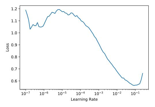
Figure 2.5: An example of a loss against learning rate plot for a range test. A good choice for learning rate in this case would be around  $10^{-2}$ .
