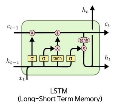
Figure 2.6: The LSTM layer. The symbol  $\sigma$  denotes the sigmoid function. Image by
