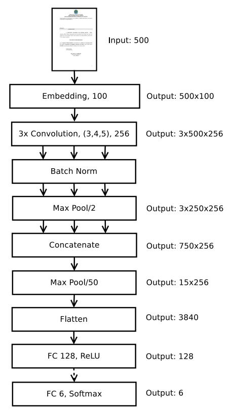
Figure 4.6: CNN architecture for document type classification. The dashed line indicates dropout was applied.
