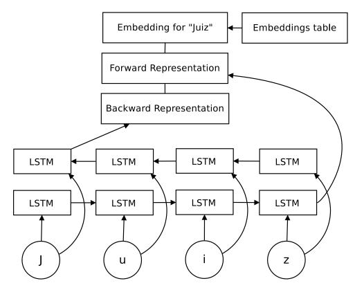
Figure 3.1: Each word vector representation is a result of the concatenation of the outputs of a bidirectional LSTM and the word level representation from the word lookup table.
