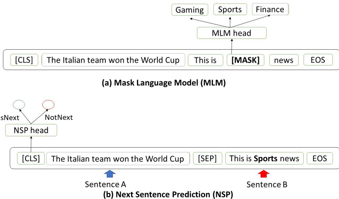
Figure 2.11: BERT [16] (a) Masked Language Model and (b) Next Sentence Prediction objectives. BERT operates over sequences of discrete tokens comprised of vocabulary words and a small set of special tokens: [CLS], [MASK] and [SEP]. The first token of every sequence is always a special classification token [CLS]. The special token [MASK] masks a word that will be predicted. [SEP] is a special separator token.
