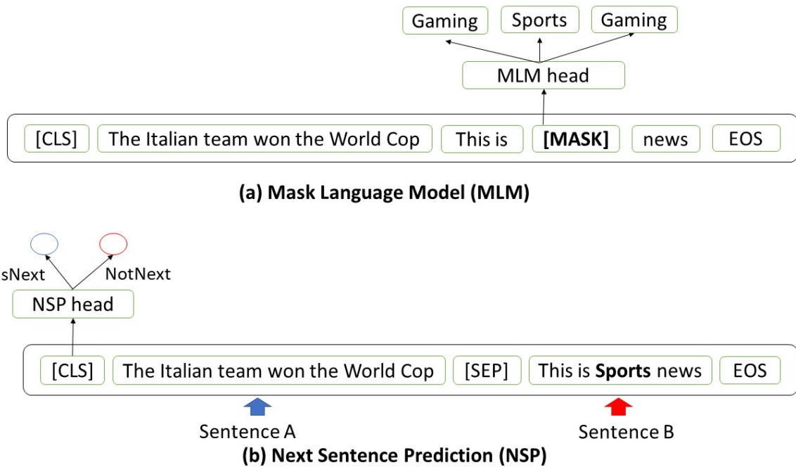
Figure 2.10: BERT [16] (a) Masked Language Model and (b) Next Sentence Prediction objectives. BERT operates over sequences of discrete tokens comprised of vocabulary words and a small set of special tokens: [CLS], [MASK] and [SEP]. The first token of every sequence is always a special classification token ([CLS]). To mask a word that will be predicted, the special token ([MASK]) is used. ([SEP]) is a special separator token.
