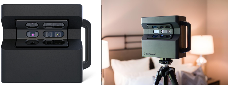
Figure 1.2: Matterport 360° Camera. This tripod-mounted device contains three structured light sensors pointing slightly up, straight ahead and slightly down. To cover the whole scene, the camera rotates around its vertical axis while captures multiple high quality RGB-D images. Source: www.matterport.com . ©Matterport, Inc. Reproduced with permission.
