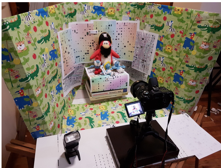
Figure 2.4: Single camera setup for stereo emulation.
