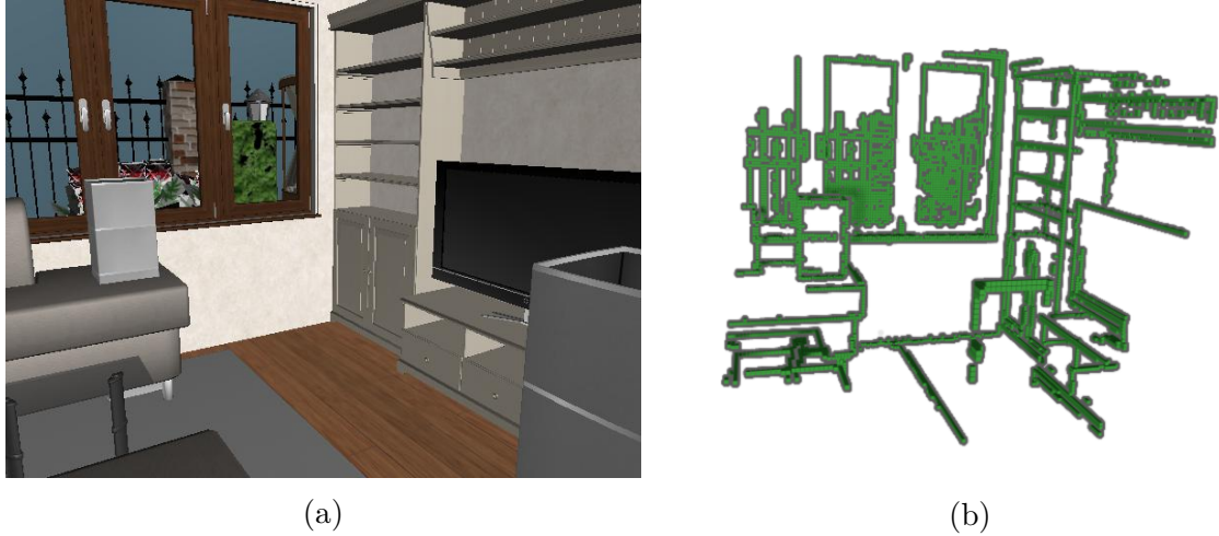
Figure 4.1: Projection of Edges to 3D: (a) original RGB image, (b) voxelized edges after projection.
